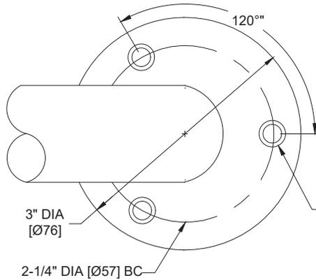
9/32" DIA [Ø7] HOLES WITH .40" DIA [Ø10.2] X 82° COUNTERSINK TO ACCOMMODATE #10 [M5] FLAT-HEAD SCREWS OR 1/4" [M6] PAN-HEAD SCREWS
