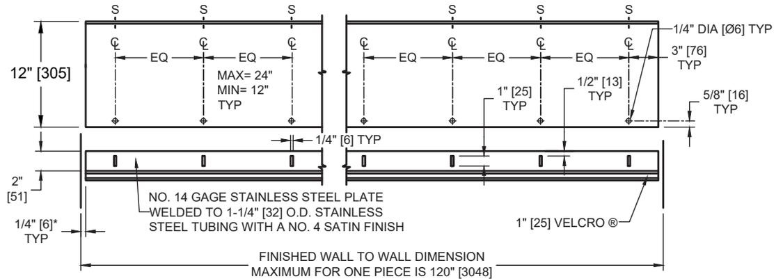
\*UNIT SHALL BE 1/2" [13] LESS THAN WALL TO WALL DIMENSION
