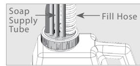
NOTE: The Multifeed Kit enables soap distribution for up to six (6) soap dispensers simultaneously. When installing less than a full complement of soap dispensers, make sure to insert and clamp the 5/16" dia x 1" long (Ø8x25) plugs into the remaining empty holes.
