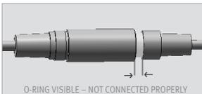
NOTICE: If the 4 contacts connectors are not connected properly, the motor will run continuously.
