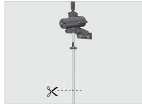
Make sure the end of the tubes are about 1" (25) longer than required to reach the tank bottom.
