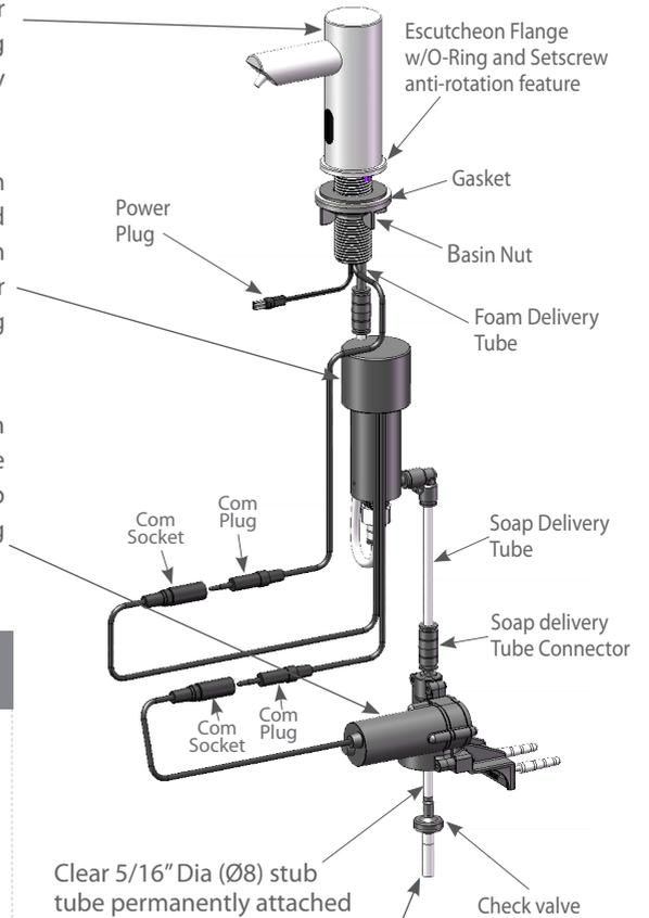
Clear 5/16" Dia (Ø8) stub tube permanently attached to pump housing, into which check valve is inserted. {IMPORTANT: Note flow direction}
