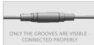
**Important:** the 4 contacts connector should be inserted fully so that the white O-ring is not visible and a clicking sound is heard.
