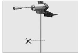
Make sure the end of the tubes are about 1" (25) longer than required to reach the tank bottom.
